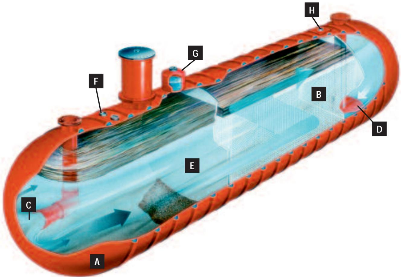
**A. Xerxes Separator:** The separator is rustproof and requires no cathodic protection.
